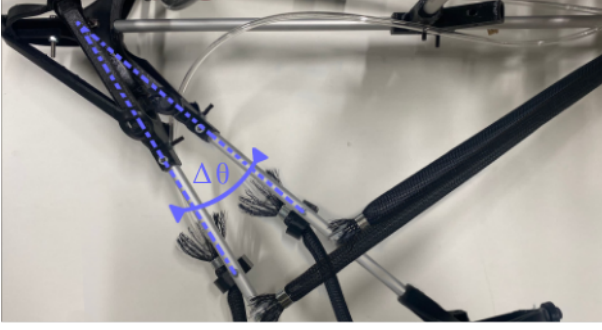
Fig. 18: Actuation effect on joint's angle
